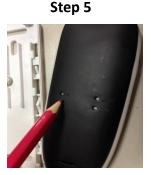
Press the "P2" button twice on the remote control using a pencil.
