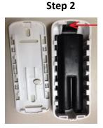
Release the tab and remove control panel from housing. Step 3
