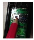
Using a pencil, press the "mode" button once on the control panel.
